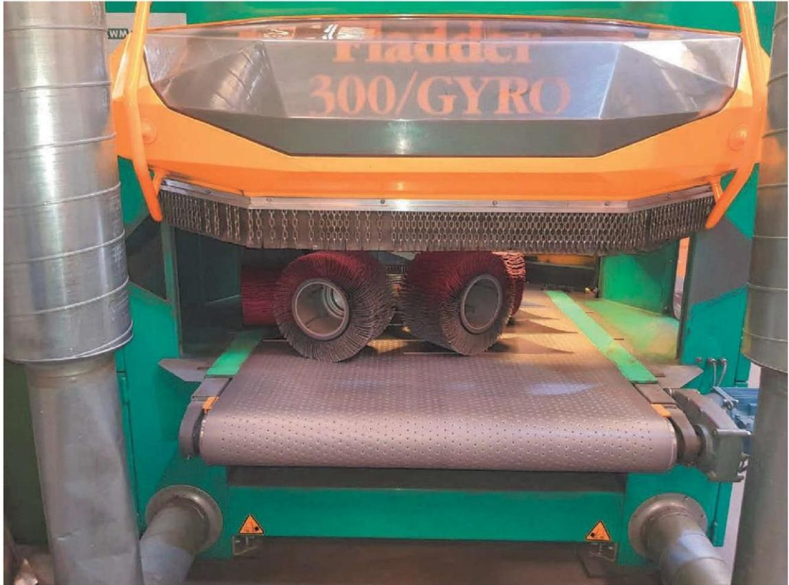
***Photograph 2: KWM Weisshaar uses the deburring roller 400x250x200mm from boeck on the FLADDER deburring machine, thus saving 50% of the machining time.***
