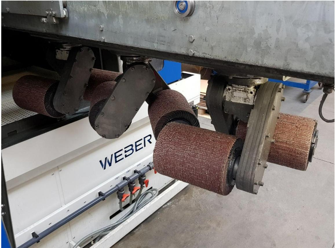
***Photograph 2: GEWA uses deburring rollers which were specially developed for wet machining.***
