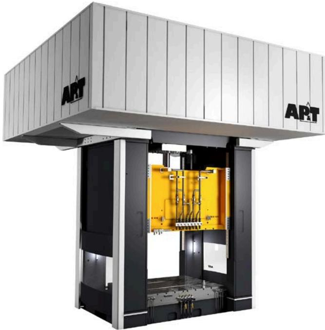
*AP&T's servo hydraulic press is not only quicker and more energy efficient than conventional hydraulic presses, it is also a powerful alternative to servo mechanical presses.*
