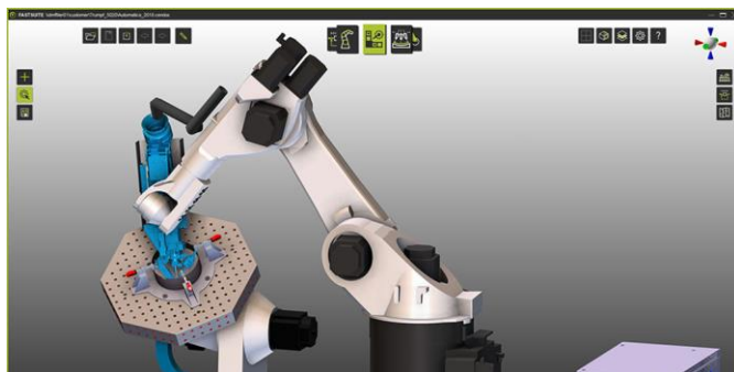
Simulation of the 3D laser welding process with the TRUMPF TruLaser Robot 5020
