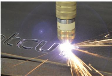
**Picture:** Kjellberg-SilentCut.jpeg – Cutting of mild steel with reduced the sound pressure level with Silent Cut
