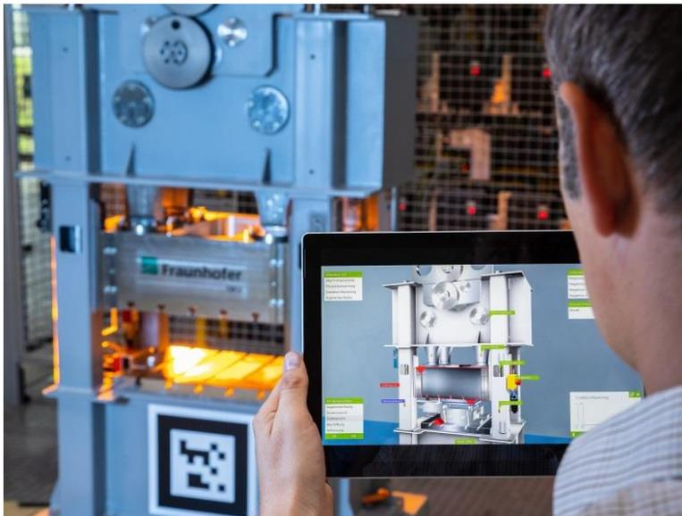
**"Forming 4.0": Uninterrupted monitoring of processes and machines can be achieved by digitization of sheet metal forming, which can significantly increase machine availability as well as service life, and considerably reduce tool setup times. | © Fraunhofer IWU**
