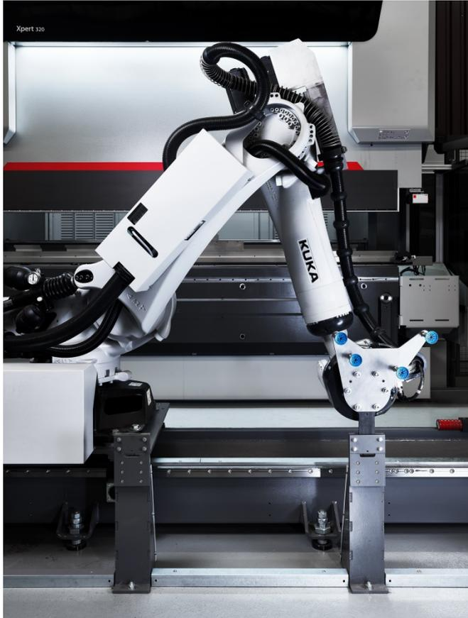
Flexible and autonomous: The 7-axis robot can handle lifting capacities up to 270 kilograms and can autonomously change grippers and bending tools.
