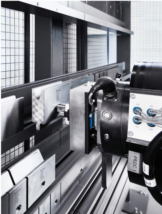
Flexibility for changing orders: With a capacity of 37 meters, the tool magazine offers sufficient space for a wide range of bending tools.
