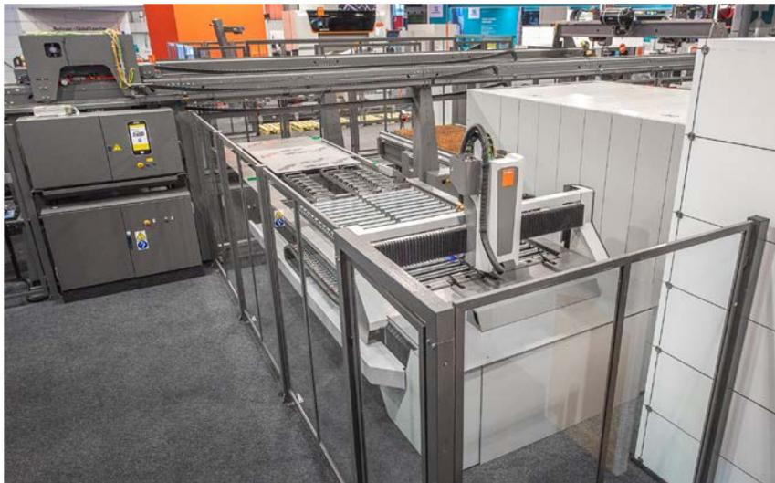
The integrated ByFlex system drills and deburrs holes, and cuts threads and countersinks into sheet metal parts prior to the laser cutting process.
