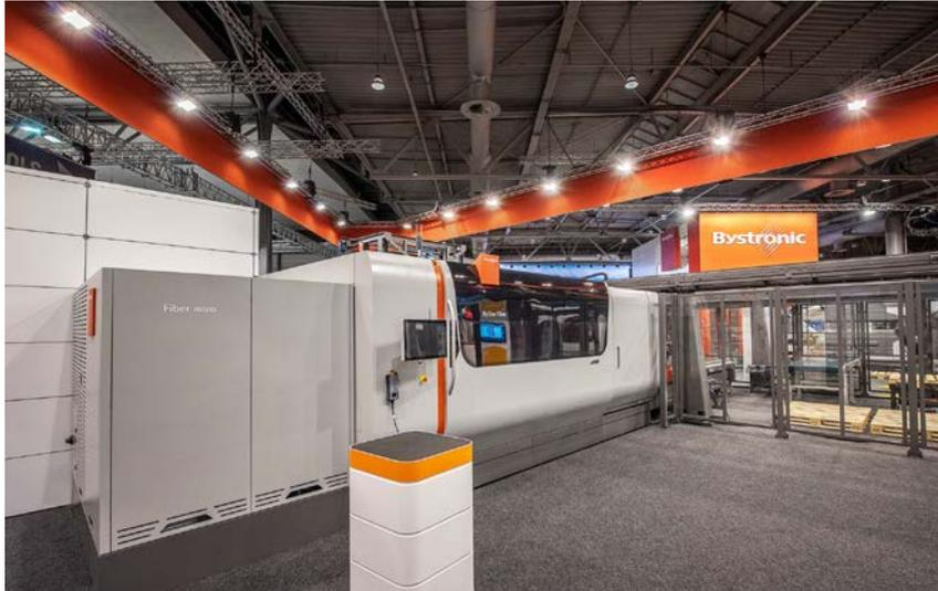
The ByStar Fiber is the heart of the Production Line. The fiber laser system is equipped with a powerful 10 kilowatt laser source.
