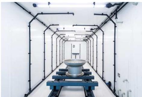
*A glimpse into Sientop's Rotainer pickling system: the components are sprayed with the bath pickle in a closed container system.*
